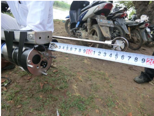
Setting of current meter (KENEK) and turbidity meter (JFE Alec).
