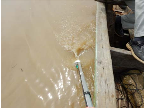
Measuring river flow and turbidity
